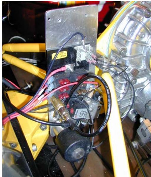
The Air Valves for the Clutch, Transmission, and Clutch Purge Note the lower large air valve rated to handle the 250 PSI CO 2 required to shift the transmission.
