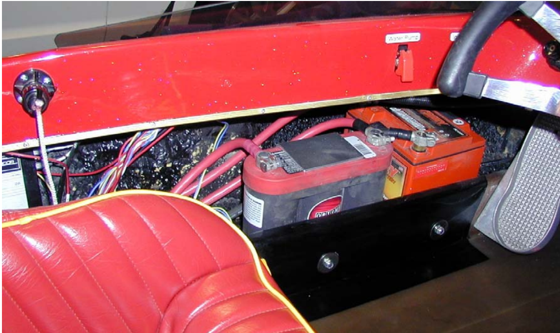
The 6V Battery (Aft) and the 12V Battery (Foreward) Located in Port Sponson
