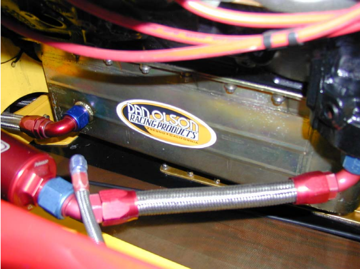
The 13 Qt Oil Pan and Wet Sump Input/Output Hose Connections
